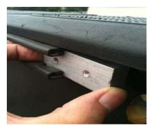
\*Attach the clamp bracket to the plate with the included allen head bolts.
