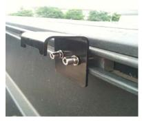
\*Line the bracket up with the tri-fold hard cover clamp location once they are lined up. Secure bracket to the vehicle bed rail. \*Secure Tri-fold Cover latches to these brackets
